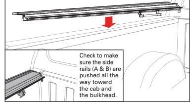
For the best (A) fit, the side rails (B & C) should be level with the truck bed cap and not angled up or down. Insert the backside of the clamp as high as possible and tighten clamp. Depending on model the notch will vary. Tighten all clamps to 10 ft/lbs of torque with a 1/2" wrench or socket. **Caution: Do NOT overtighten!**
