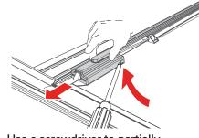
Use a screwdriver to partially pry open the tab on the latch housing. At the same time slide the housing away from the latch assembly.
