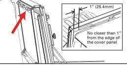
**16** Unfold the cover (A) towards the tailgate. Then confirm each panel is centered side to side and front to back on the truck bed. If adjustments are needed, loosen the cover retainer clamps (G) and shift the cover until positioned correctly. The rear edge of the cover and tailgate seal should rest on top of the tailgate. For proper sealing, the tail panel will overlap by .5".
